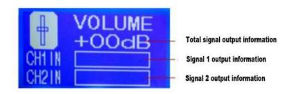
Turn on and enter the main interface, turn the multi function key to adjust the total volume. During the process, the total signal output, signal 1 output and signal 2 output will have corresponding information changes.
