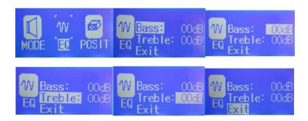
Under menu ,place the cursor to EQ and then enter sub menu when you turn left and right multi function, Choose Bass or Treble to add or reduce volume. Turn left turn right multi function to move the cursor on Bass,press multi function, the cursor will place on Bass data adjustment, then you turn multi function left or right to add or reduce data, when you set up
